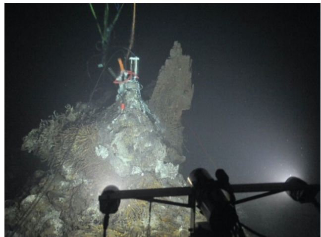
The RCA cabled digital still camera, redeployed in 2015 by the Canadian ROV ROPOS, lights up the active hydrothermal vent called El Gordo in the international District Hydrothermal Field, located at the summit of Axial Seamount nearly a mile beneath the ocean surface. Credit: UW/NSF-OOI/CSSF.
